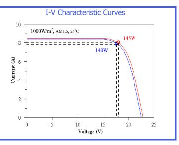
Electrical specification are based on measurements performed at standard test conditions (STC) of 1000 W/m² irradiance, air mass 1.5 and cell temperature of 25°C after long-term stabilization. Performance may vary up to 10% from rated power due to temperature operation, spectrum and related effects.
